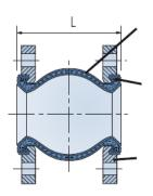
Body of synthetic rubber and reinforcing fiber.
