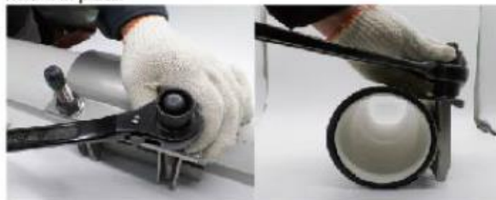
Step4 Use a tension wrench to sequentially tighten the studs to the recommended tension specified on the clamp.
