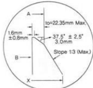
BEVEL FOR WALL THICKNESS(to) 0.88" IN.(22.35mm) OR LESS.
